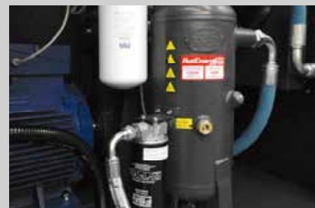
**Oil filter and oil separator filter**
